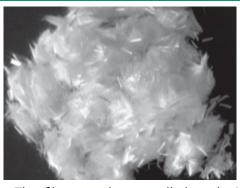
The fibers work as small threads / micro-reinforcement tying up the concrete particles, This reduces the cracking caused and also increases the tensile strength of concrete
