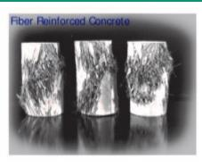
FiberCrete also gives protection from explosive spalling incase of fire and helps maintain the structural integrity.
