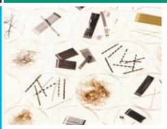
FiberCrete contains micro fibers for added tensile strength, better binding ability, resistance to cracking & abrasion
